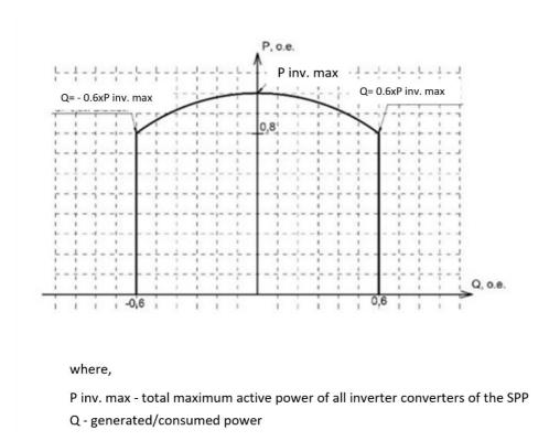
Figure 4. Dependence of SPP's Reactive Power Regulation Range on Its Actual Generation
