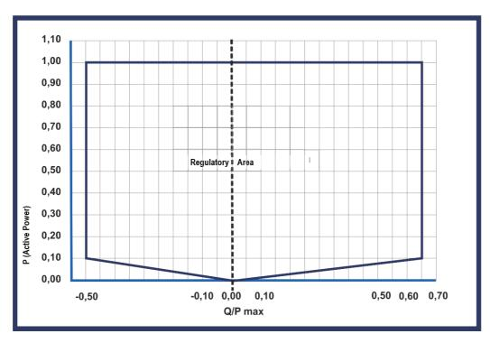
Figure 6. Dependence of SPP's Reactive Power Regulation Range on the Actual Voltage at the Connection Point
