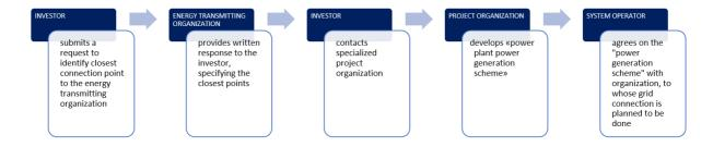
Figure 3. Procedure for Identifying the Closest Connection Point and Developing the Power Plant Power Generation Scheme
